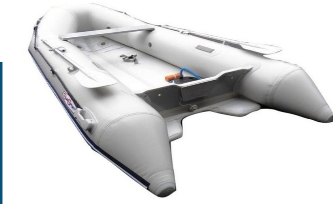
Three Chamber System All SunSport models have a maximum of 3 air chambers.
